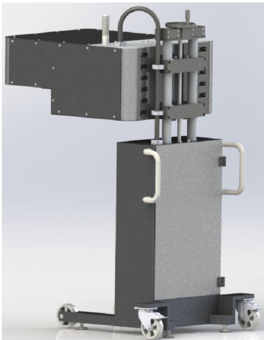
In addition, a height adjustment in z of 300mm was needed to adjust the focus to the workplace, as the unit is to be used in several positions. The complete electrics and electronics should be located within the desired unit.
